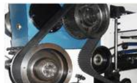
Timing belt drive, Intermittent mechanism
