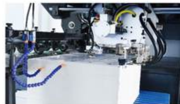
Feeder (4 suction and 6 feed)
